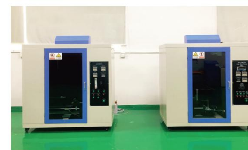
Needle Flame Testing Machine
